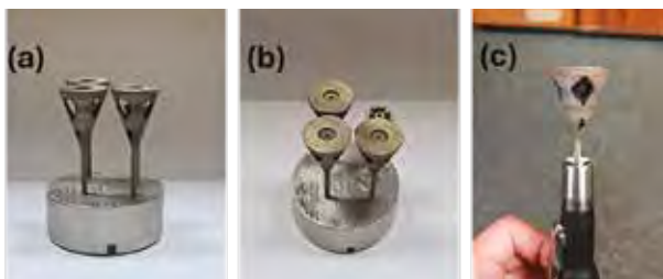
3D printed polishing tools for laminated engineering materials and the 3D printed part fitted to the polishing machine.
