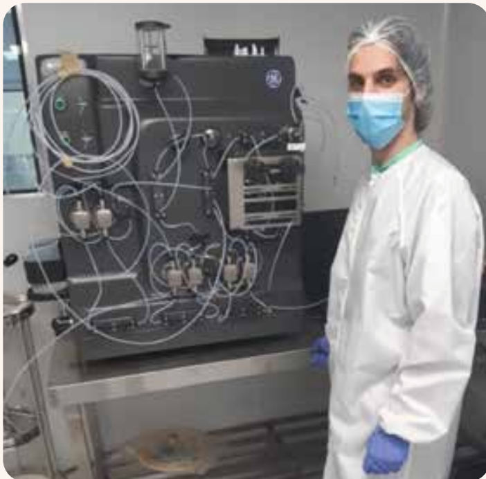
Figure 17: An Altis Biologics employee operating a high-end fast protein liquid chromatography system
