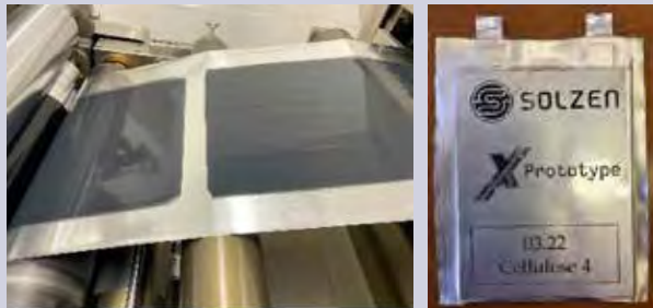
Figure 7: Production of The Solzen ultracapacitor, showing the prototype being made (left) and the final prototype produced (right)
