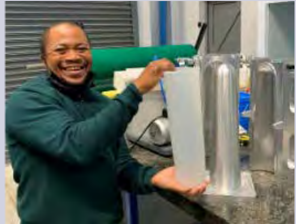
Figure 28: Luvuyo Sume with a silicone prosthetic liner and the tooling for injection moulding the liners
