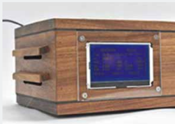
A low-cost air quality monitor that measures levels of air pollution in the air and has been used in houses across South Africa.
