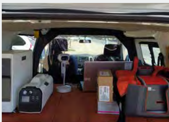
Panel van set-up with portable point-of-care (POC) tools for screening of TB, HIV, and diabetes.
