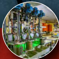
Bacterial cultures are maintained in the laboratory for ore leaching
