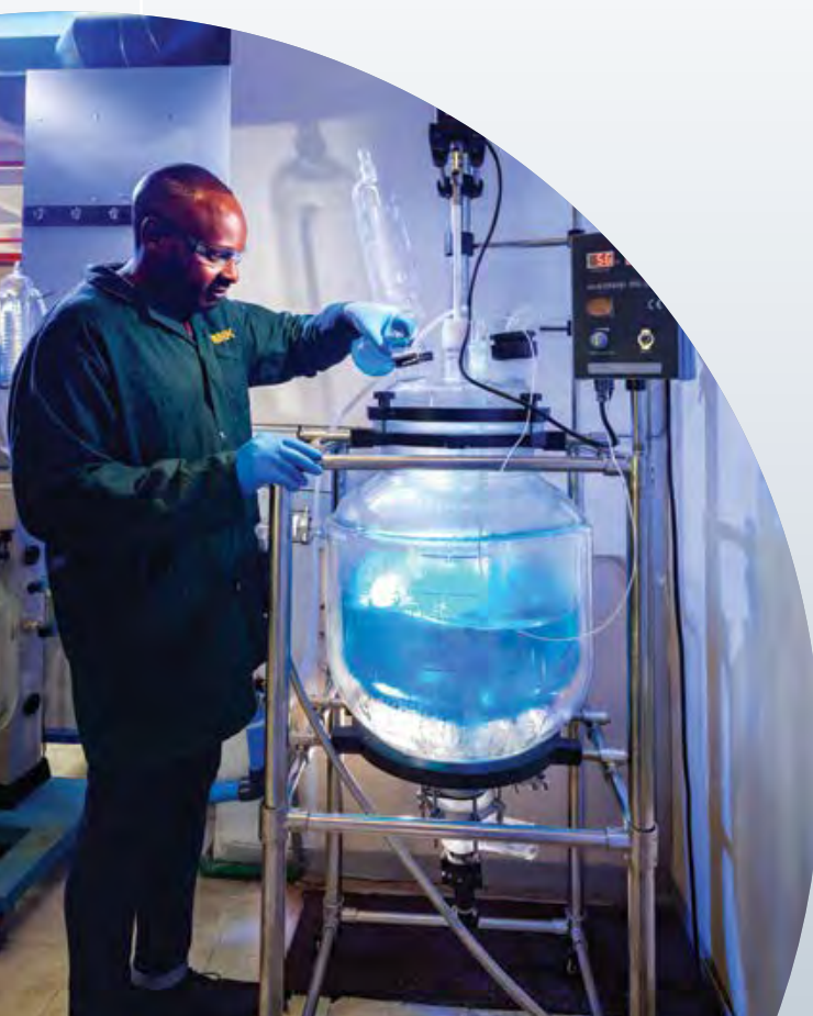
Left: A jacketed glass reactor is used for the upscaling of powder modifications
