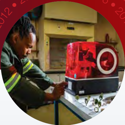
A 3D printer is used in the design and prototyping of moulds in jewellery making.
