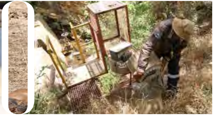
Collecting boundary stream water from an autosampler
