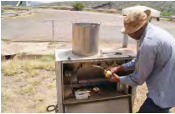
Fallout pots and air sampler to sample airborne particulates
