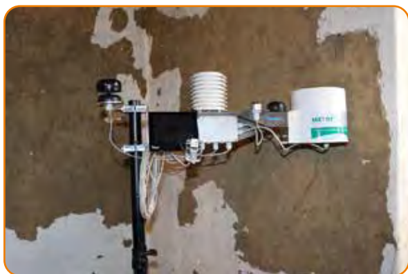
Figure 16: Climate Smart localised weather station developed under the Eureka Climate Smart Agriculture project
