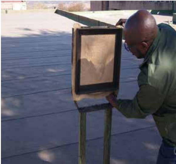
Tacky sack deployment to monitor air particulate fallout. Monitoring streams leaving the Pelindaba site.
