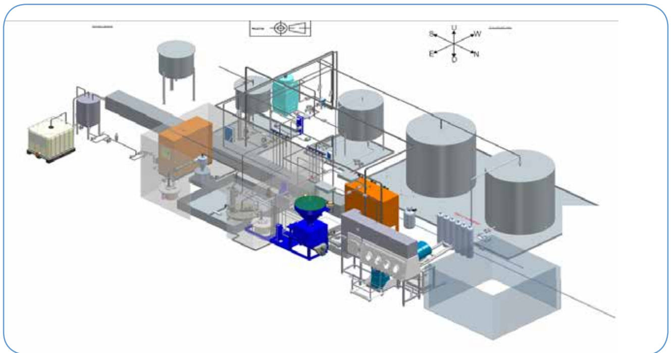
Nuclear Waste Plasma Gas Plant (Solid Waste & Oil)
